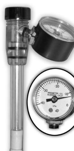
**The IRROMETER Body** — is constructed of tough durable plastic impervious to attack by soil chemicals or electrolysis.
